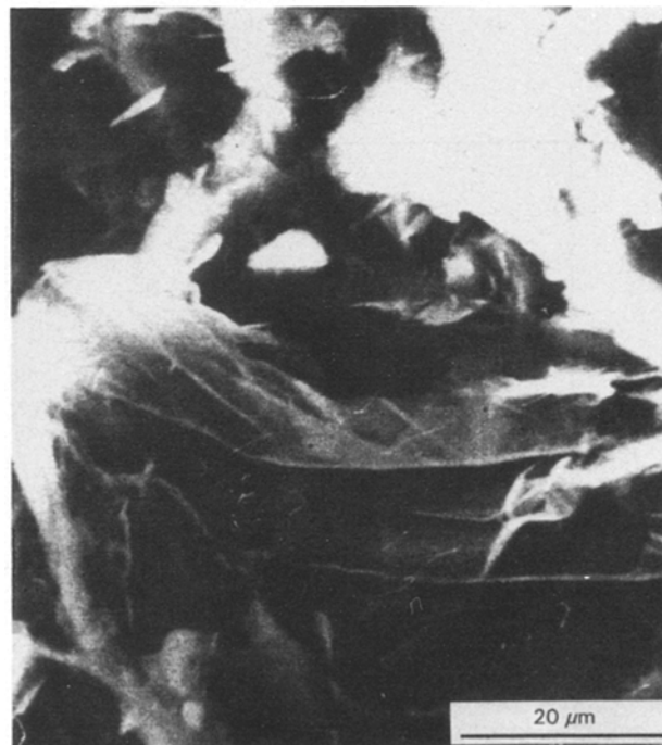
Figure 3 SEM photomicrograph of the graphite-epoxy surface.
